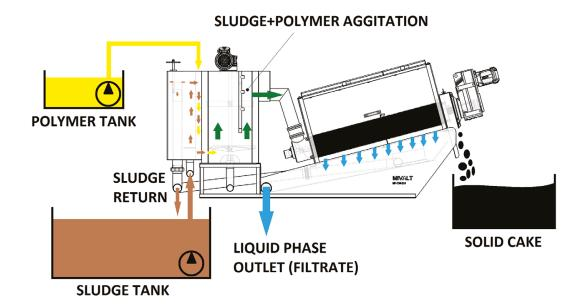
De-sludged water returns to the wastewater treatment plant, where it can be biologically treated. Sludge which is discharged from the end of the machine can be transported, for instance, by means of a belt conveyor. Dewatering substantially reduces sludge volume, thus reducing transportation and disposal costs.
