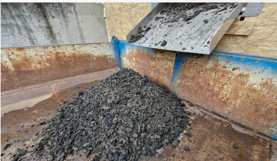
Dewatered cake from MP-EDW
